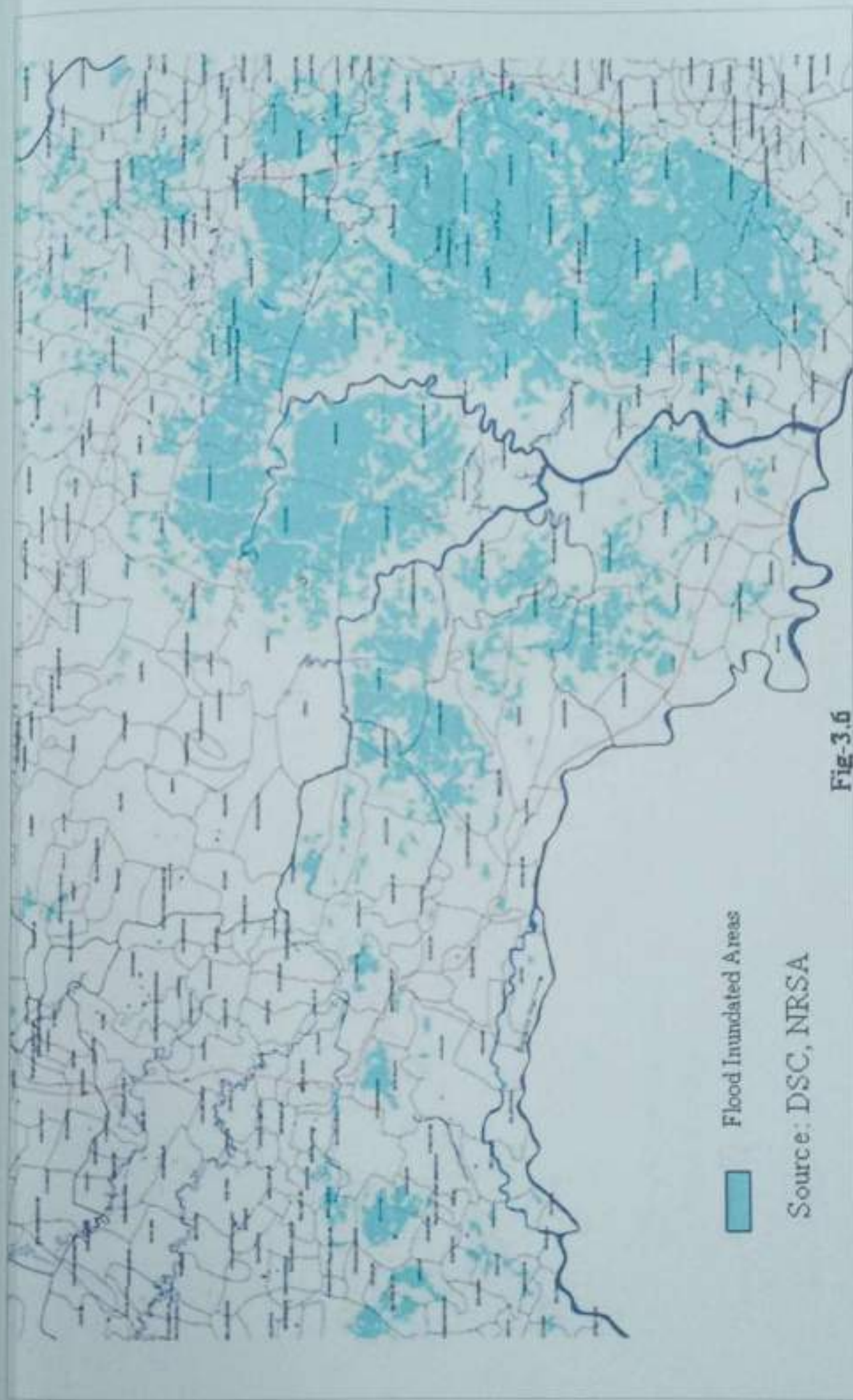
Flood Inundated Areas in part of Bhadrak District, Orissa Based on the Analysis of Radarsat data of 13 th July 2007
